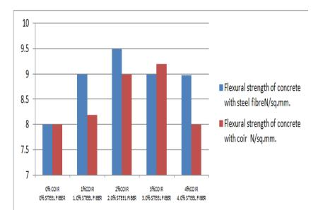
Addition of coir by 2.0% & 3.0% considerably increase the flexural strength as compared to the steel fibers.
